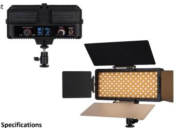
Color temperature: 3200K – 5600K Beam angle: 120° Color rendering: > 90 LED life: approx. 30.000 hours Power draw: approx. 15W Power input: Battery: Sony NP-F, Panasonic AG-VBR or Canon LP-E6 Mini XLR-4: 5V DC to 18V DC
